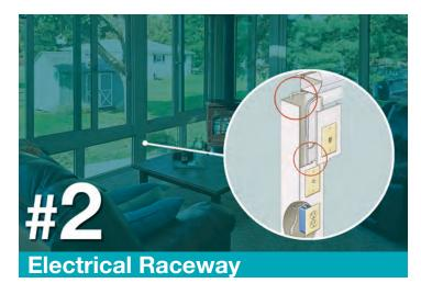
The electrical raceway allows you to add interior or exterior electrical features to your sunroom, such as phone lines, cables and speakers.
